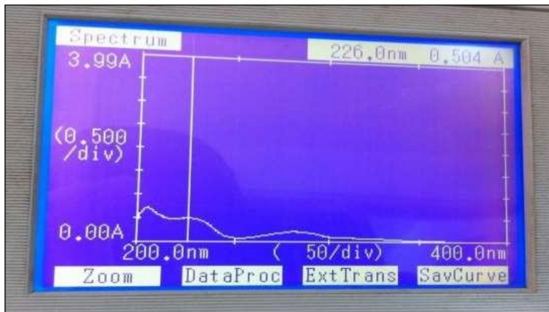
Figure 4.3: Absorption spectrum of Glabridin in ethanol
